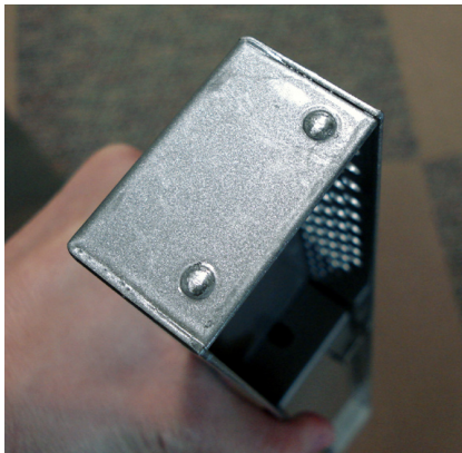
Fig. 2 - Bumps on right end of bezel
